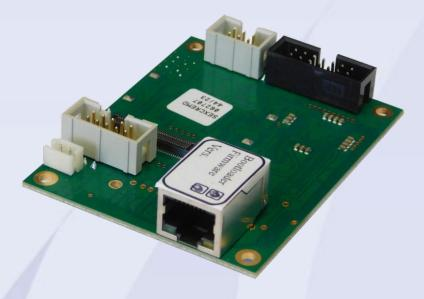
SEXC30REMD and SEXCREMD+ are optional interface cards that allow remote control via the Internet or LAN network of equipment and systems (of any type) produced by Sielco. The SEXC30REMD+ version is also equipped with a modem for GSM data connection\*\*.
